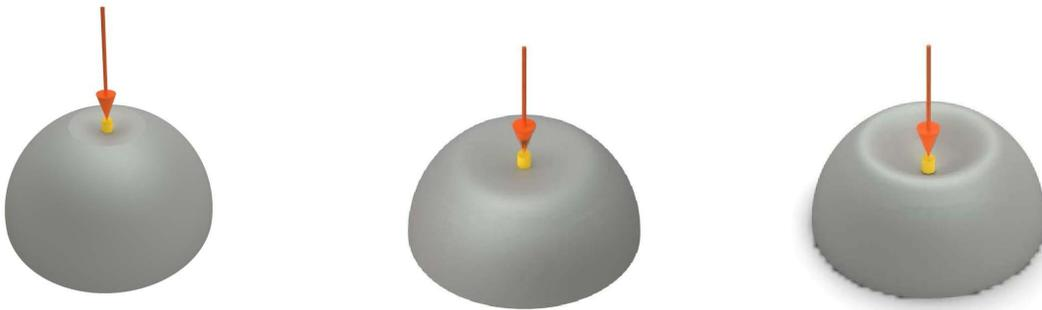
Fig. 1. Geometry of post buckling of hemispherical shells subjected to concentrated load
