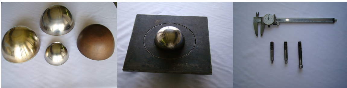
Fig 2. Different size of bosses, hemispherical shells and rigid support used for experimental study
